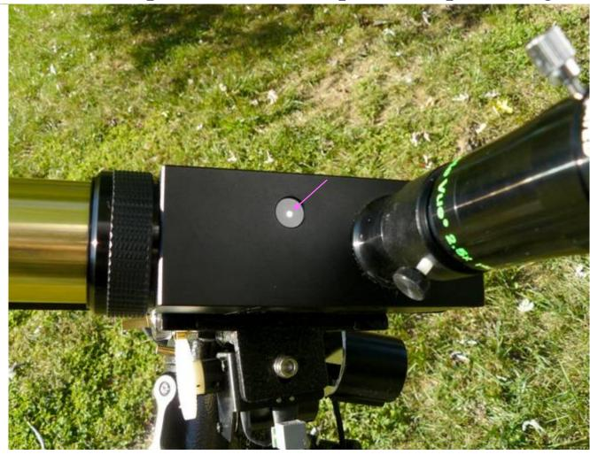
Do the final fine adjustments using the RA and DEC controls to center the sun. If large adjustments is needed, tracking will be less than optimal, so it may be best to start fresh, trying to eliminate errors to minimize inaccuracies.
