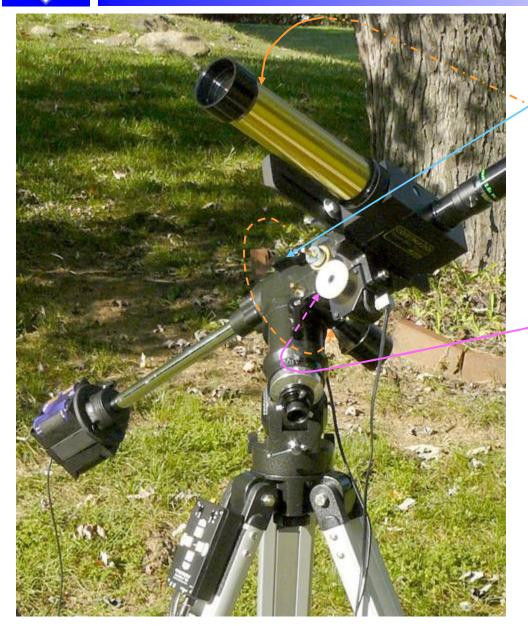
(a) Loosen the DEC clutch,
