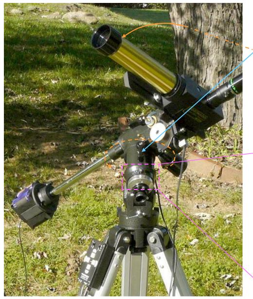
(a) Loosen **RA clutch**, and <u>push the scope</u> over so that the RA setting circles indicates the sun's RA position (13:12 in this case). Re-tighten the RA clutch.
